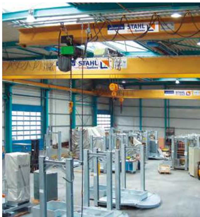
The single-fall design of the ST 50 chain hoist permits fast hoisting speeds for load capacities up to 2,500 kg. It is mounted with a push trolley on a wall slewing crane.
