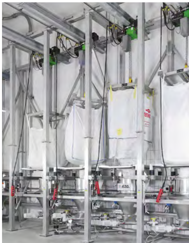
Big bag beams are lifted up to top hook position without any hindering edges with the big bag design for load capacities up to 3,200 kg.
