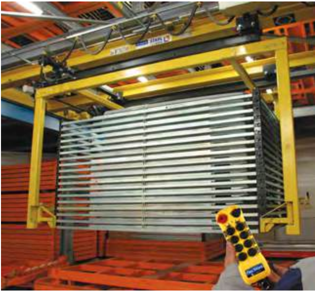
Two STD dual chain hoists with the aid of four synchronously operating load hooks enable long goods weighing 10 tonnes to be transported without swinging.
