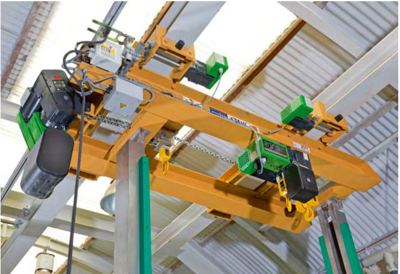
A special crane with height-reduced suspended crane endcarriages and an individually adapted custom hoist works in a chemical plant in Germany. The custom hoist is an STD 50 dual chain hoist with two synchronised rope lead-offs. An ST 20 chain hoist serves as an auxiliary hoist.
